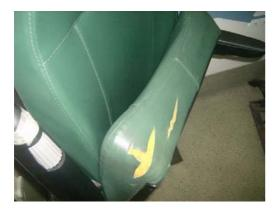
2.30 The chairs in the patient area of both of the vehicles were found to be torn, allowing fluids, dirt and bacteria to penetrate the material. These should be re-covered or replaced with an impermeable material so that they can be clean appropriately.
