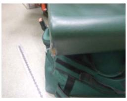
2.47 In three of five vehicles chairs within the patient area were found to be torn, allowing fluids, dirt and bacteria to penetrate the material. These should be re-covered or replaced with an impermeable material so that they can be clean appropriately.
